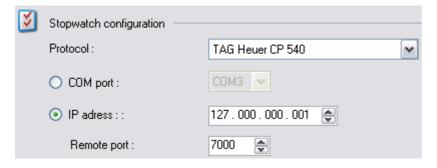
The IP address **127.0.0.1** is a special purpose address reserved for use on each computer. 127.0.0.1 is conventionally a computer's *loopback* address. Network software and utilities can use **127.0.0.1** to access a local computer's TCP/IP network resources.
